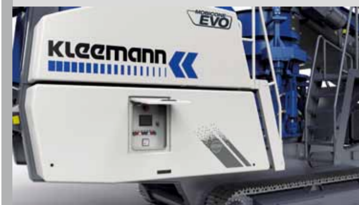
Easy accessibility with separate flap in control cabinet
