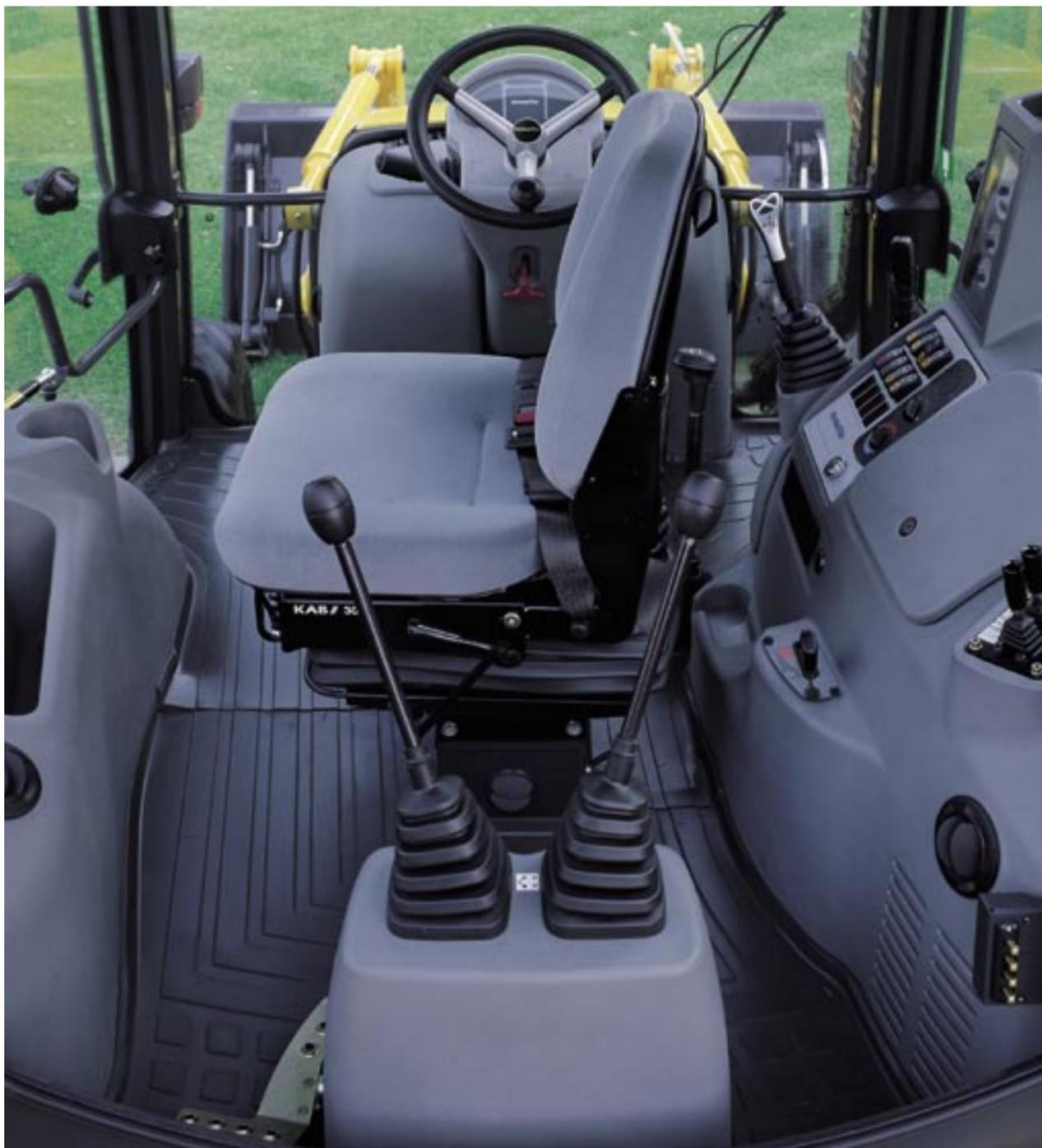
With a ROPS and FOPS structure and a modern design, the cab features a top class automotive style. Its increased internal volume and wide round glass surface offer great comfort to the operator. The optimal air distribution maximizes the ventilation system and the optional air conditioning system, which include ten conveniently located vents. Complete instrumentation, easily reachable control panel and plenty of holders and storage compartments make this machine the best in its class.
