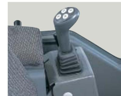
Automatic transmission is used with joystick steering.
