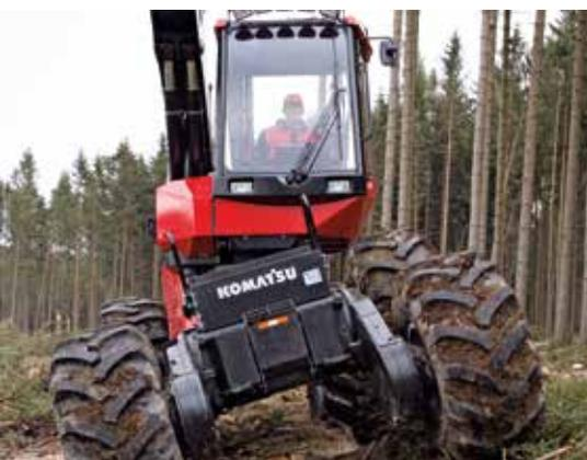
Cab and boom leveling and stabilizer coupling for superior stability and ground contact.
