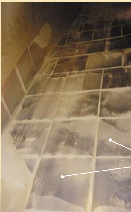
Grizzly bar caps installed on an iron ore grizzly screen (right).
