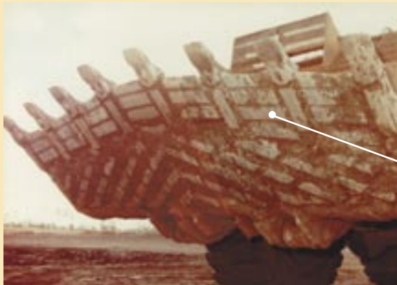
Grizzly bar caps installed on an iron ore grizzly screen (right).
