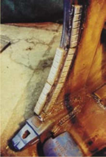
Wear bar and "chocky" bar configuration on bottom of dragline bucket (right).
