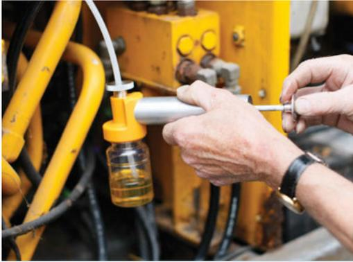
Oil sampling is at the heart of condition monitoring. These handy kits allow hydraulic oil samples to be taken safely. All kits include analysis from a leading laboratory and a simple to interpret cleanliness report to ISO 4406.
