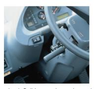
Easy shifting and directional changes with Komatsu two-lever electronic shifting. Change direction or shift gears with a touch of the fingers without removing the shifting hand from the steering
