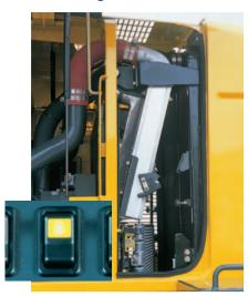
If the machine is operating in adverse conditions, the operator can reverse the hydraulic cooling fan from inside the cab by turning on a switch on the control panel. The coolers can also swing out for easy cleaning.
